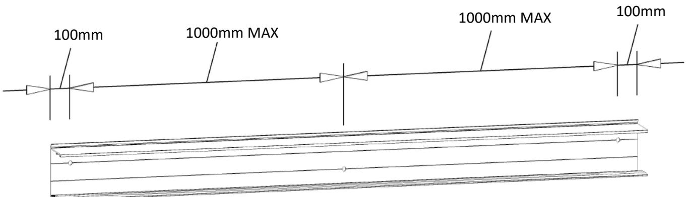
For 10mm  $\emptyset$  holes use alternate drill positions 1 & 2
