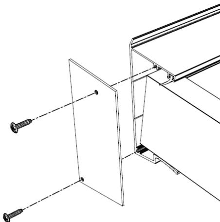
Apply silicone to gutter edges before fitting end plate.
