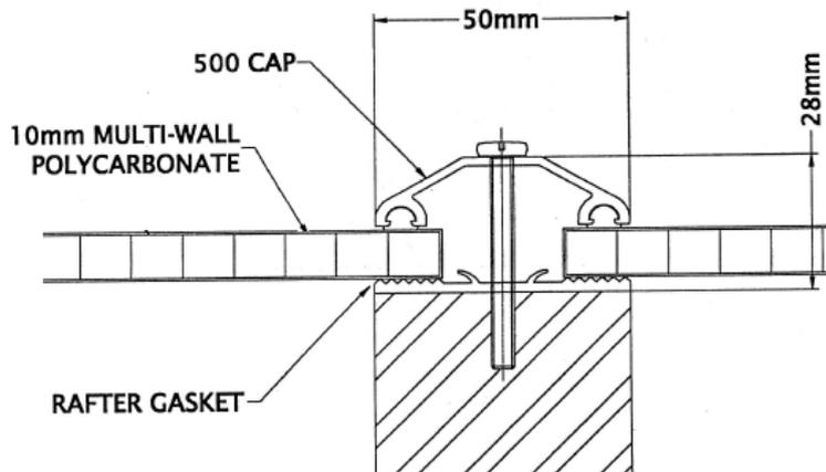
The P501 system is used to install multiwall polycarbonate or glass ranging from 4mm to 25mm onto 50mm wide rafters. The P501 is supplied as a pre-pack complete with aluminium cap, gaskets and end plate.
